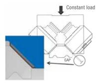
When a heavy load is applied, the rollers are free to flex until the carriage body leans on the guide, discharging on it all the load that otherwise would break the rollers. After removing the load the carriage is again able to move regularly on the rail.
